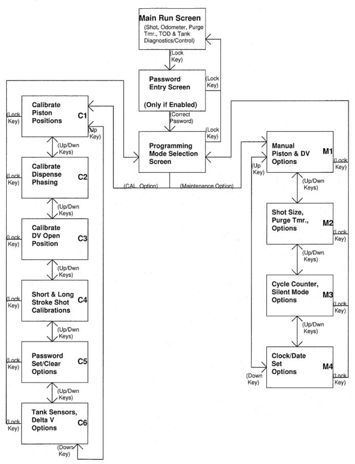
Figure 9: PR70 Screen Navigation Diagram
